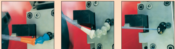
TYPE 1 OddBall attached to 1/4" Loc-Line* hose. TYPE 2 OddBall attached to 1/4" Snap-Loc** hose. TYPE 3 OddBall threaded onto 1/8 NPT/BSPT TurretJet.
